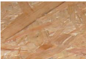
OSB - Oriented Strand Board
